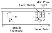
Figure 3 - Electric Stove Control Panel
